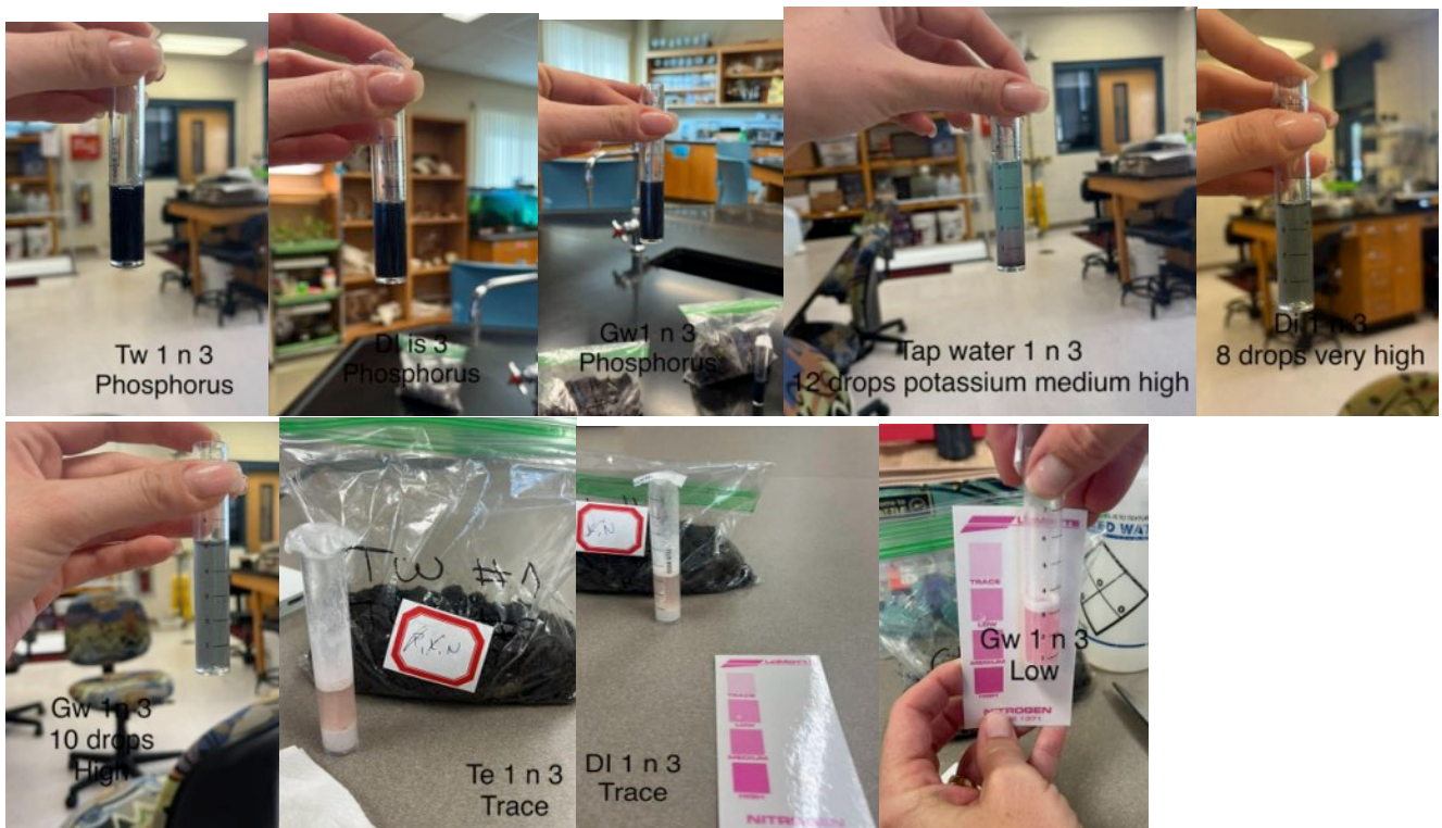
Figure 4. Colorimetric results for (a-c) P, (d-f) K, and (g-i) N. In each series, treatments are tap water, DI and greywater.
